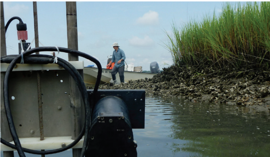
Imaging sonar systems provide opportunities to count, measure, and characterize movements of fishes and motile invertebrates (nekton) in turbid waters. Identification to species is not always possible and the field of view is limited; however, deployments in intertidal salt marsh creeks have revealed patterns of tidal movements, feeding behavior, predator-prey interactions, and other activities
