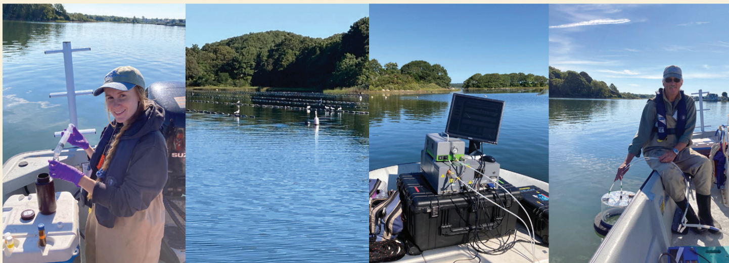
Team members, Zan Beardwood and Don Cobb, sampling water and greenhouse gases in Rhode Island salt ponds. A floating chamber set by Don Cobb was used to measure greenhouse gases. The Picarro gas analyzer in the boat simultaneously measured carbon dioxide, methane, and nitrous oxide
